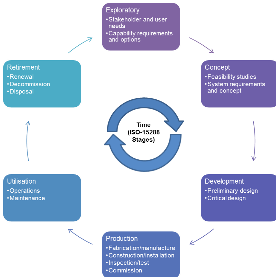
Figure 2: Asset life-cycle phases of ISO/IEC 15288-2008
