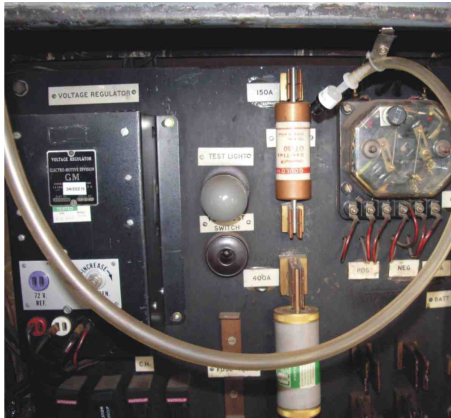
Cabin fuse & battery knife switch backing board in a Y class locomotive
