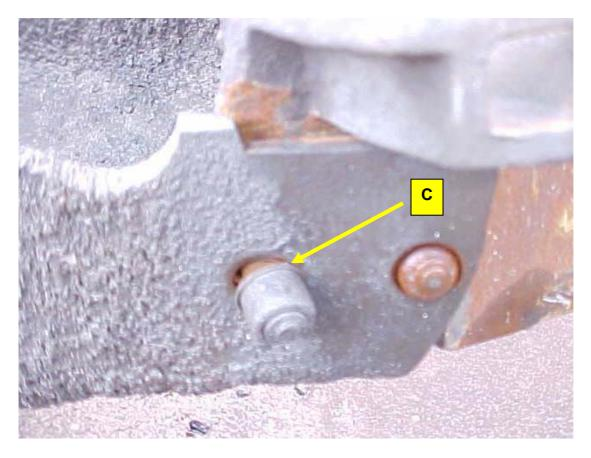
Arrow C in photograph 2 indicates to a loose / worn rivet (huck bolt) on a Knorr break beam of a CQMY wagon, which is the subject of this safety alert.
