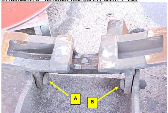
Arrows A & B in photograph 1 indicate to the subject rivets (huck bolts) on a Knorr brake beam of a CQMY wagon.
