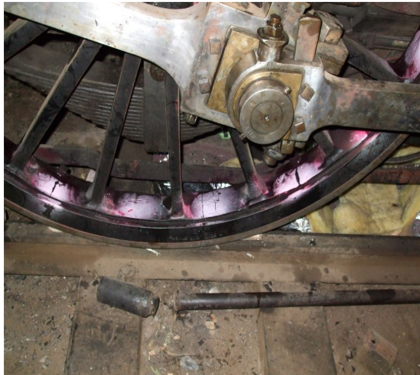
Figure 1 – Inner wheel rim surface showing transverse fractures on several segments
