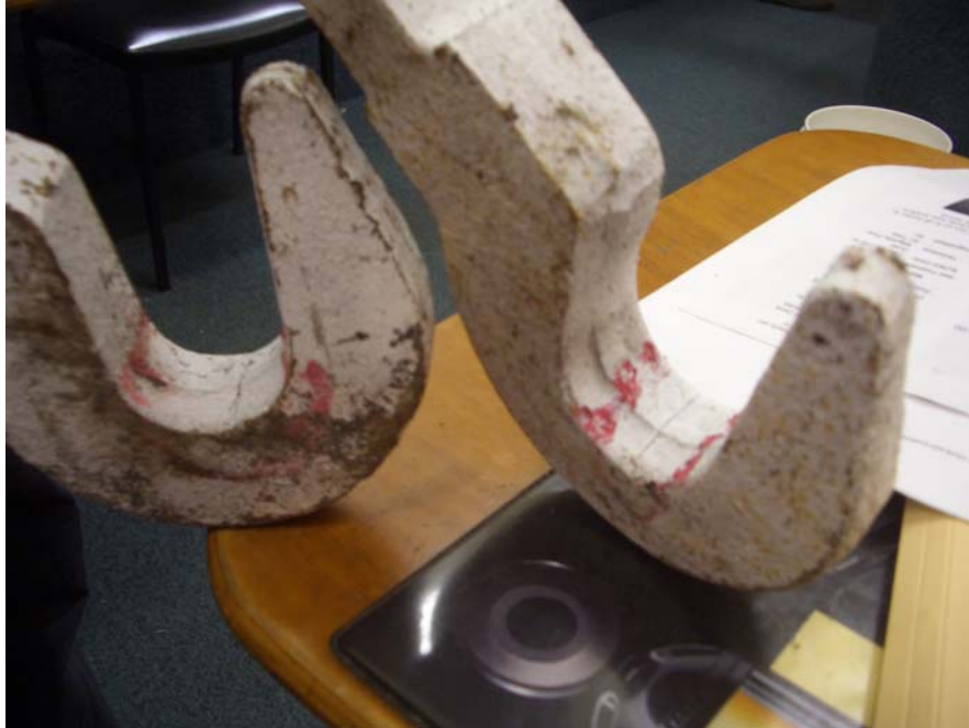
Figure 3 - Two drawhooks showing fractures on the inner contact surface
