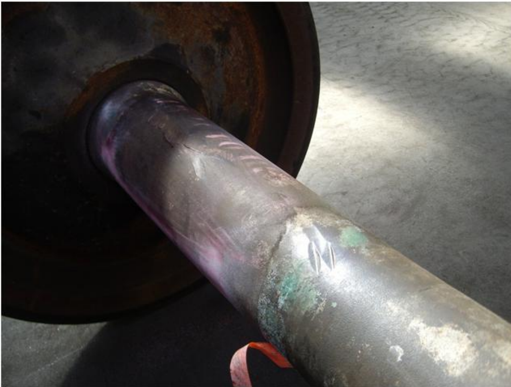
Figure 7: Axle D, heavy impacts marks evident after the identification tape had been partially removed.
