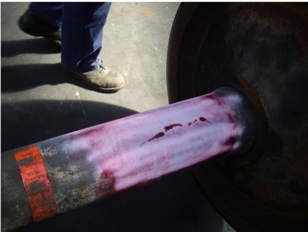
Figure 6: Axle D, significant abrasion marks. Note the identification band still wrapped around the centre of the axle.
