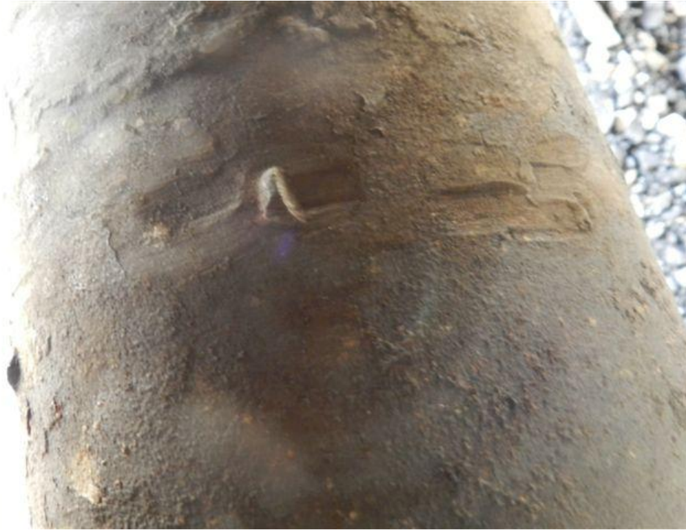
Figure 1: Axle A, heavy transverse gouge marks
