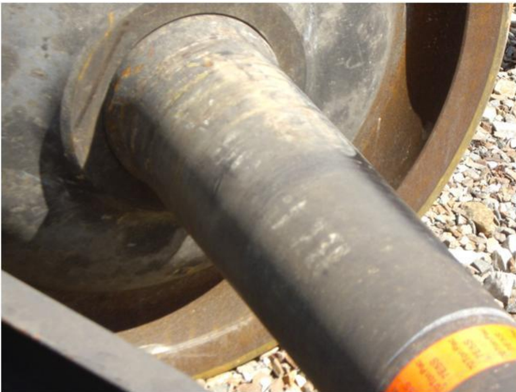
Figure 4: Axle C, transverse impact mark
