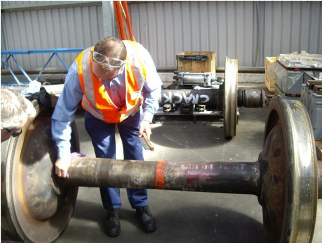
Figure 5: Axle D (foreground); Chinese-manufactured axle found with sub-surface defects (background).
