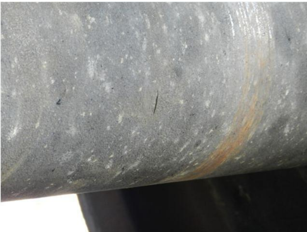
Figure 2: Axle B, small sharp transverse incision
