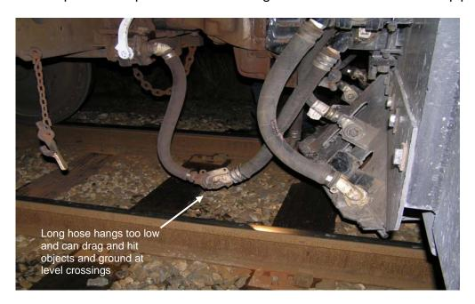
3. The potential for brake pipe isolating valve to be struck by un-restrained brake pipe hose
