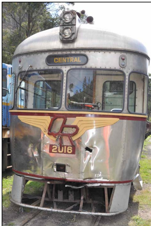
Photograph 6: Rail Motor 2016 collision damage
