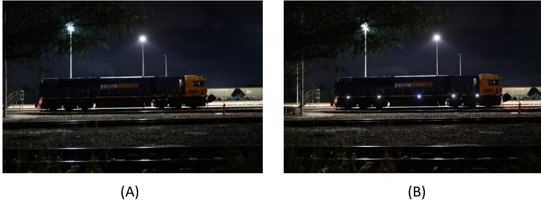
FIGURE 54. LOCOMOTIVE SIDE WITH WHITE SIDE MARKER LIGHTS (A) OFF, AND (B) ON. THE YARD FLOOD LIGHTS ARE BEHIND THE LOCOMOTIVE
