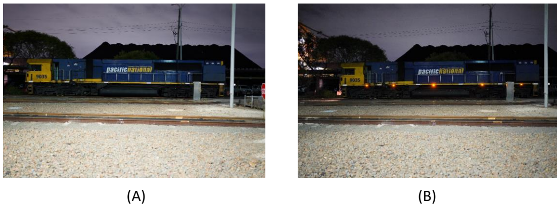
FIGURE 55. LOCOMOTIVE SIDE WITH AMBER SIDE MARKER LIGHTS: (A) OFF, AND (B) ON. NOTE THAT THE SIDE OF THE LOCOMOTIVE IS WELL-ILLUMINATED DUE TO THE YARD FLOOD LIGHT
