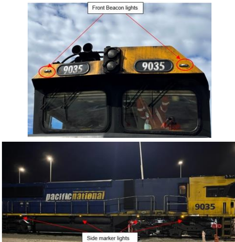
FIGURE 1. BEACON LIGHTS ON THE FRONT OF LOCOMOTIVE (TOP), AND SIDE MARKER LIGHTS ALONG BOTH SIDE SILLS OF THE LOCOMOTIVE (BOTTOM)
