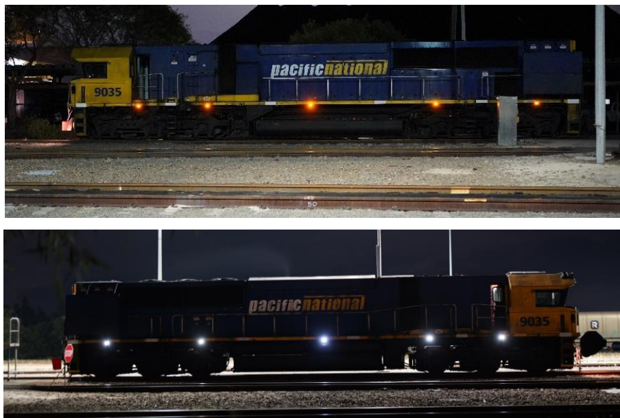
FIGURE 3. AMBER SIDE MARKER LIGHTS (TOP) AND WHITE SIDE MARKER LIGHTS (BOTTOM) ALONG THE SIDE SILLS OF THE LOCOMOTIVE
