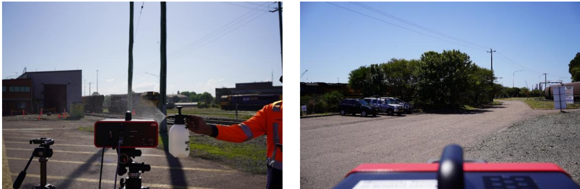
FIGURE 16. MEASUREMENT TAKEN UNDER LIGHT RAIN CONDITION (LEFT) AND VEGETATION (RIGHT)
