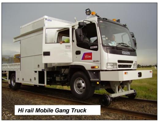
The RM Track maintenance group operates 18 'Mobile Gangs' through out the state each equipped with a set of engine powered tools
