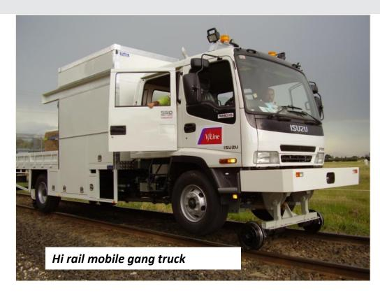
The RM Track maintenance group operates 18 'mobile gangs' through out the state each equipped with a set of engine powered tools
