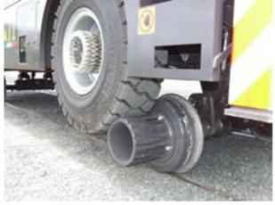
Figure 3: High ride Hi-Rail vehicle with friction drive directly on friction hub or drums fixed to rail wheels
