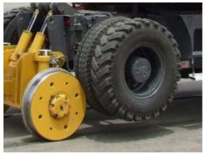
Figure 2: High ride Hi-Rail vehicle with friction drive directly on rail wheels
