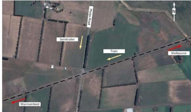
This sighting issue is exacerbated by the acute angle between the road and rail geometry, which present further challenges for road users to identify an oncoming train. It is noted in the collision report that the angle is non-compliant with level crossing design standards.
