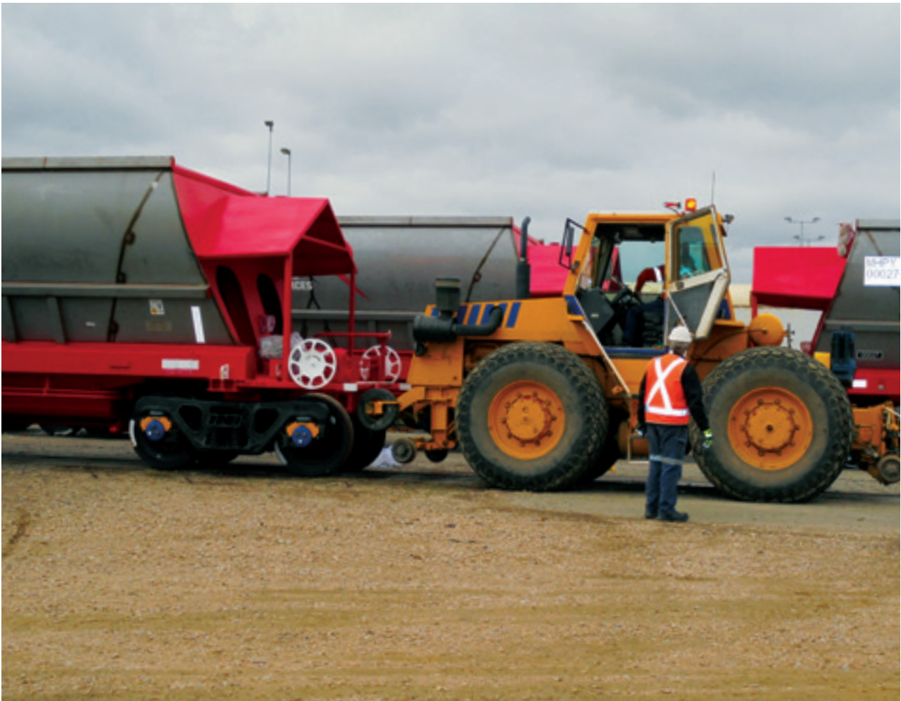
Road Rail Vehicle at Dry Creek, South Australia
