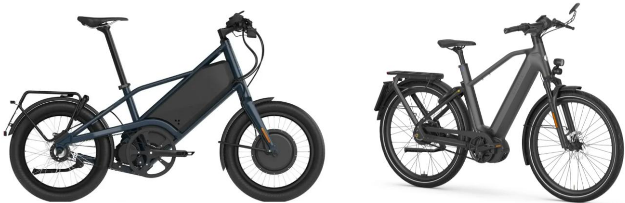
Figure 2-2: Speed pedelecs examples. Left: Ellio Original speed pedelec, 1500 W motor, speeds up to 45 km/h (Ellio, 2026) Right: Gazelle Eclipse speed pedelec, 750 W motor, speeds up to 45 km/h (Gazelle Bikes, 2026)
