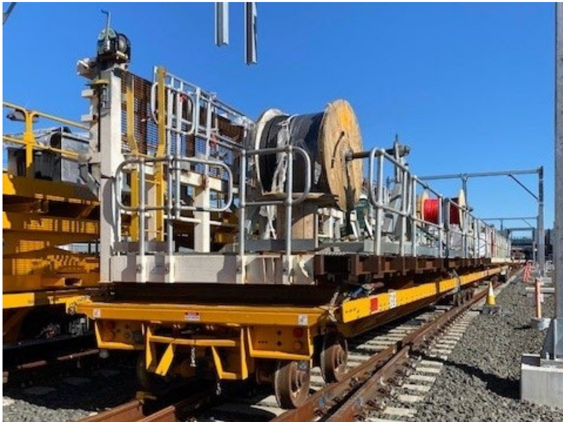
Figure 1: Runaway trailer loaded with wire coils – GVM 30t
