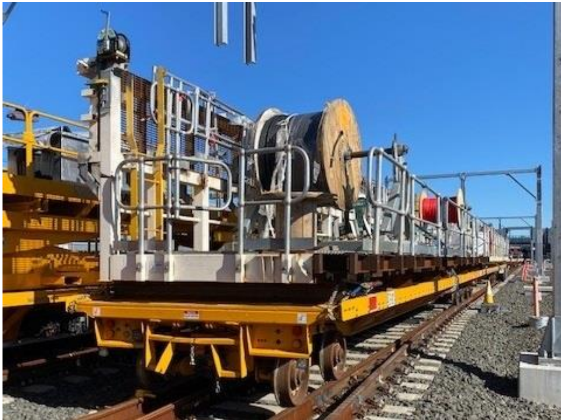
Figure 1: Runaway trailer loaded with wire coils – GVM 40t
